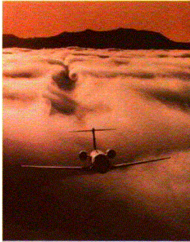
Fig 6 Downwash and wing vortices in the fog. (Photographer Paul Bowen, courtesy of Cessna Aircraft, Co.)
