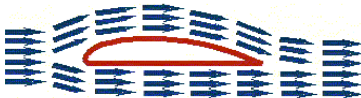
Fig 3 Common depiction of airflow over a wing. This wing has no lift.
